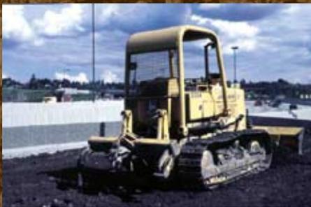
Cat-mounted rippers can break up compaction, or rip in the first lift of imported soil.
